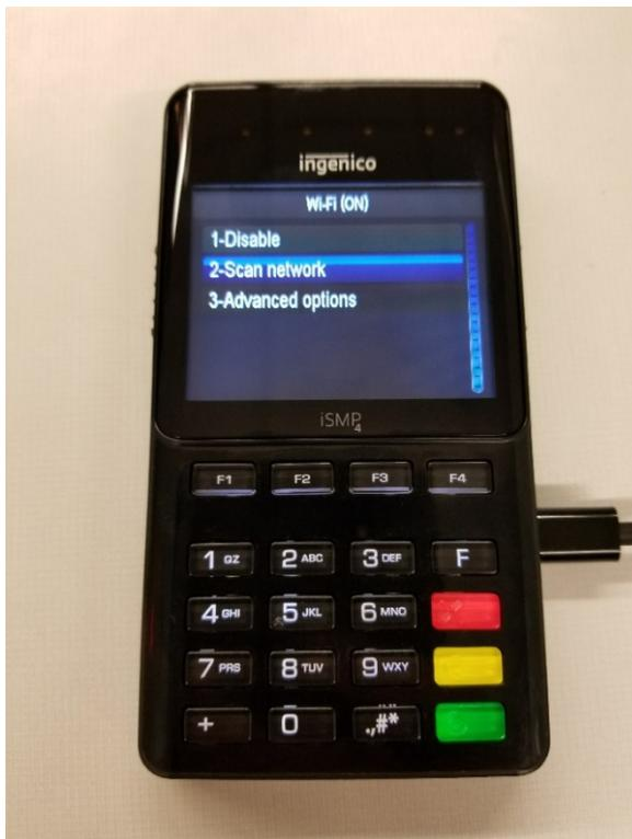
E. Select 2-Scan network to find the corresponding SSID or select "Other" if the network is hidden.
