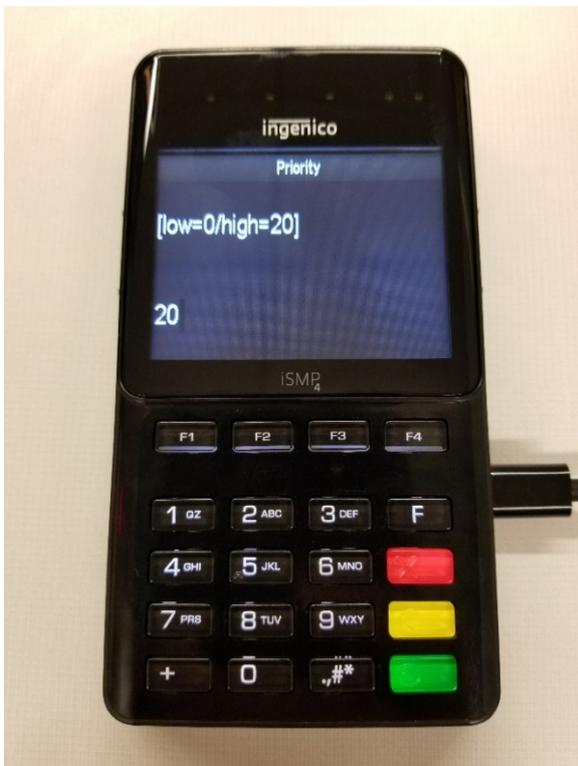
M. Priority, as to which network is used first if multiple set, will be set to 20, whether using Enterprise or Home Security. This is the final step if using Home Security.
